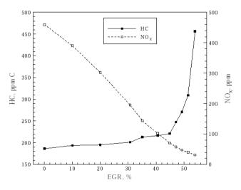
Fig 8. Trade-off between HC and NOx concentration as a function of EGR Level
