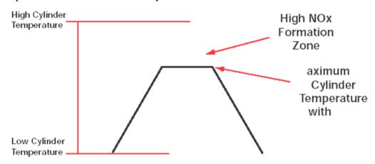
Fig 4. NOx reduction by lowering the temperature
