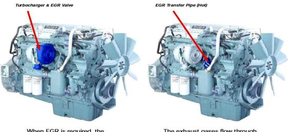
When EGR is required, the engine's electronic controls open the EGR valve.
