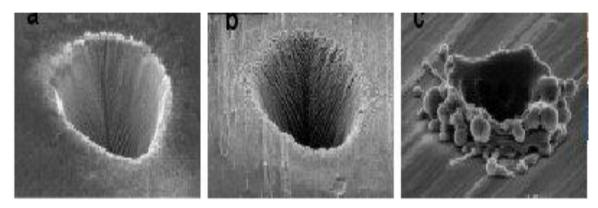
Femtosecond Laser Micromachining
