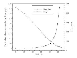
Fig 9. Relation of PM Accumulation Rate and NOx emission with EGR. Particle Size
