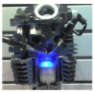
Fig.1. DTSI Engine (Courtesy: Bajaj Pulsar Bike)
