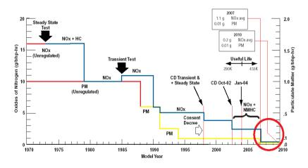
Fig 3. EPA Heavy Duty Engine Emission Standards
