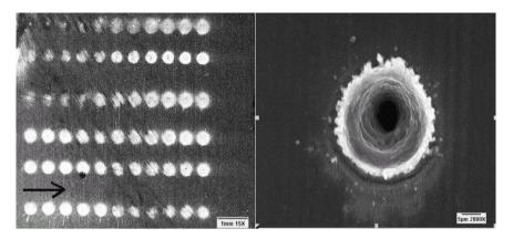
Holes drilled in 25µm thick brass foil
